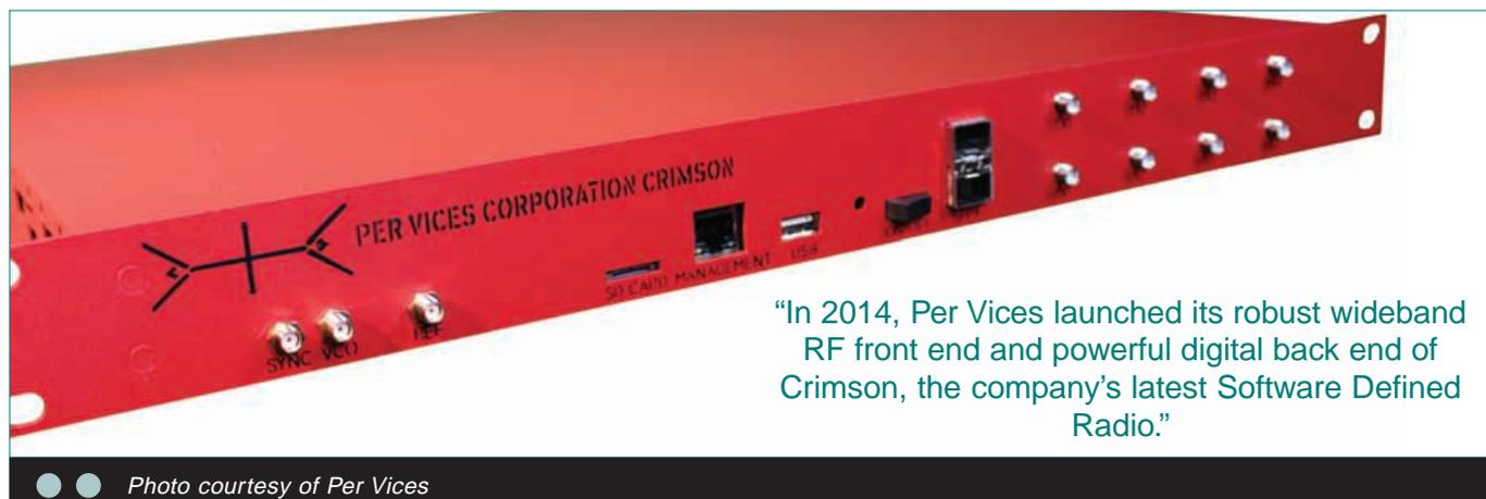
"In 2014, Per Vices launched its robust wideband RF front end and powerful digital back end of Crimson, the company's latest Software Defined Radio."
